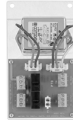
PTB → Power Termination Board
