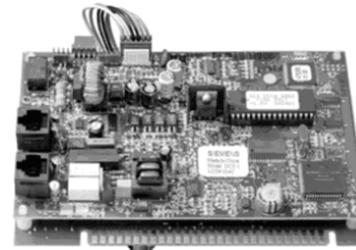
MDACT → Multi-Point Digital Alarm Communicator Transmitter
